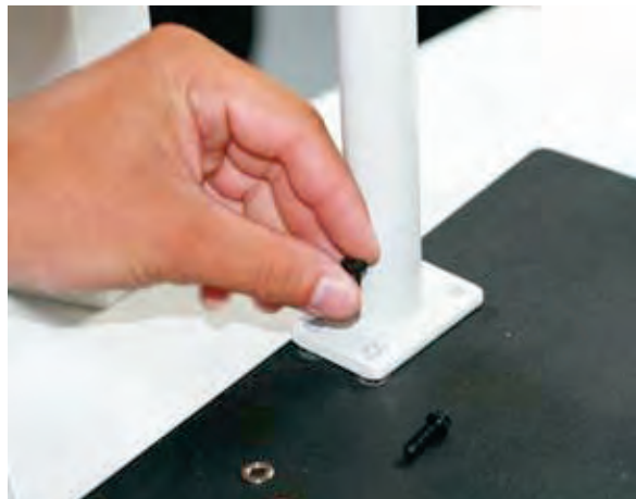
Figure 11. - Place hand post on scale platform and install screws and washers
